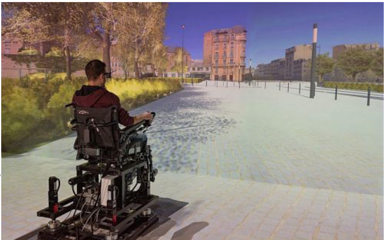
Simulator for learning to drive an electric wheelchair. The learner sits in an wheelchair facing a large screen showing an inner-city environment (Inria-IRISA Rennes 74 ).
